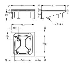
inclusive stainless steel grid with rubber bumps, with two brackets,
