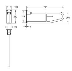
absorber, 4 mm thick mounting plate with three fixing holes, includes stainless steel screws and dowels.
