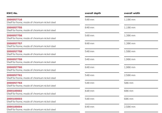
shelve for KWC commercial sinks with 600 or 700 mm depth, stainless steel, surface satin finished, material thickness 1.2 mm, inclusive shelve holder.
