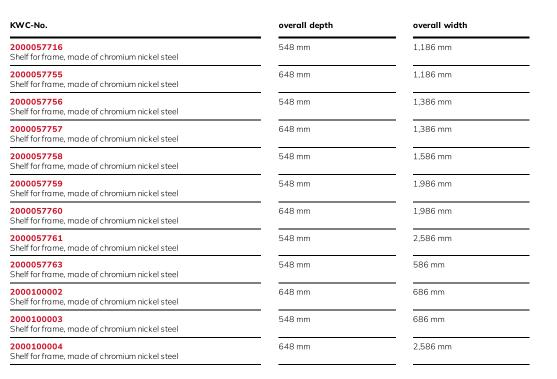
shelve for KWC commercial sinks with 600 or 700 mm depth, stainless steel, surface satin finished, material thickness 1.2 mm, inclusive shelve holder.
