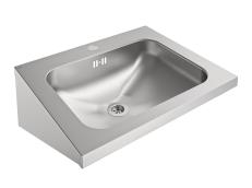
Single wash basin for wall mounting, stainless steel, surface satin finished, material thickness 1 mm, seamless welded bowl with diameter 500 x 400 x 200 mm, rectangular shape, 70 mm tap ledge, with overflow, 1 1/4" plug waste, drainage rewards centric,
