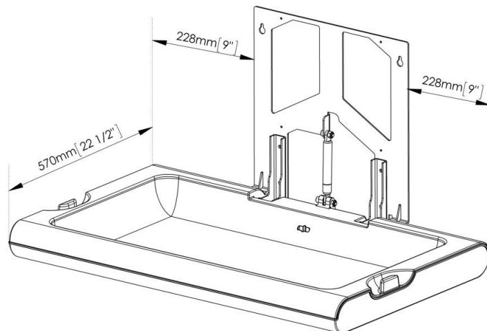
The recommended installation height is 800 mm from the ground to the lowest part of the changing station. The following sketch shows the height at which the holes should be made in order for the changing station to be installed at the recommended height:
