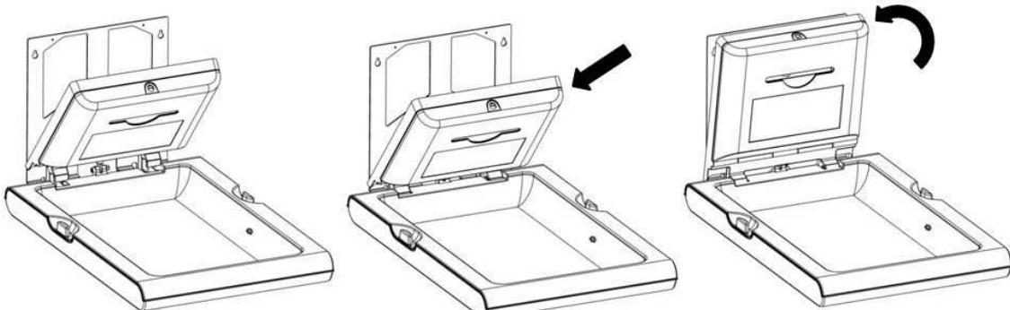
Open the liner dispenser with the special key provided. The four holes for mounting the liner dispenser on the holding structure of the changing station will be visible.
