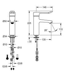
coating, in line with two-senses principle (tactile and visual). For connection to hot water and cold water via pipes, includes strainers. Tap optimised for cleaning, all-metal construction, polished
